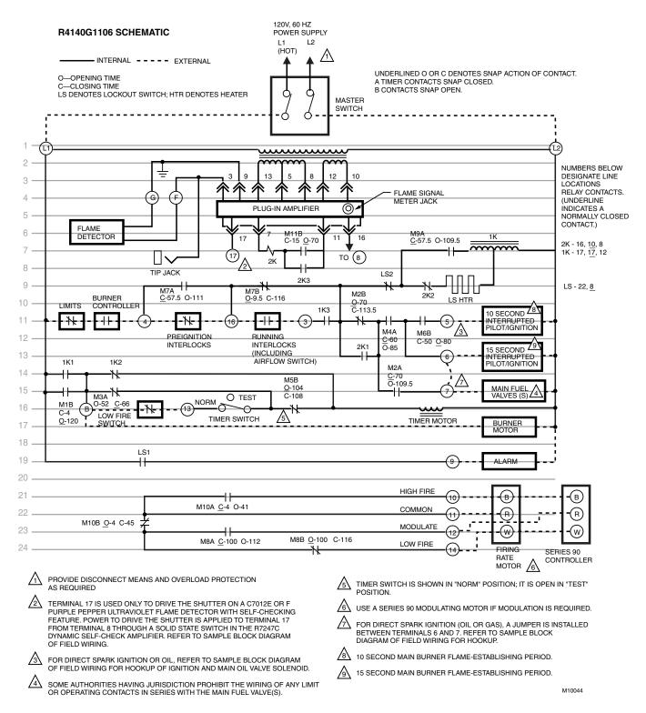
Fig. 5. Simplified schematic diagram of R4140G1106 Programmer.
